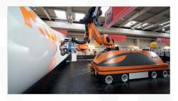
KUKA's **omiMove robot** is designed to move heavy loads across a factory autonomously, such as trains and large aircraft parts, again responding to a pull command from the assembly station that needs the large component for fit out.
